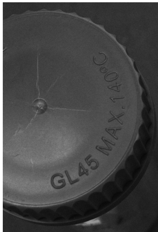
Fig. 4. Failed accelerated aging vessel showing fractures on the screw cap
